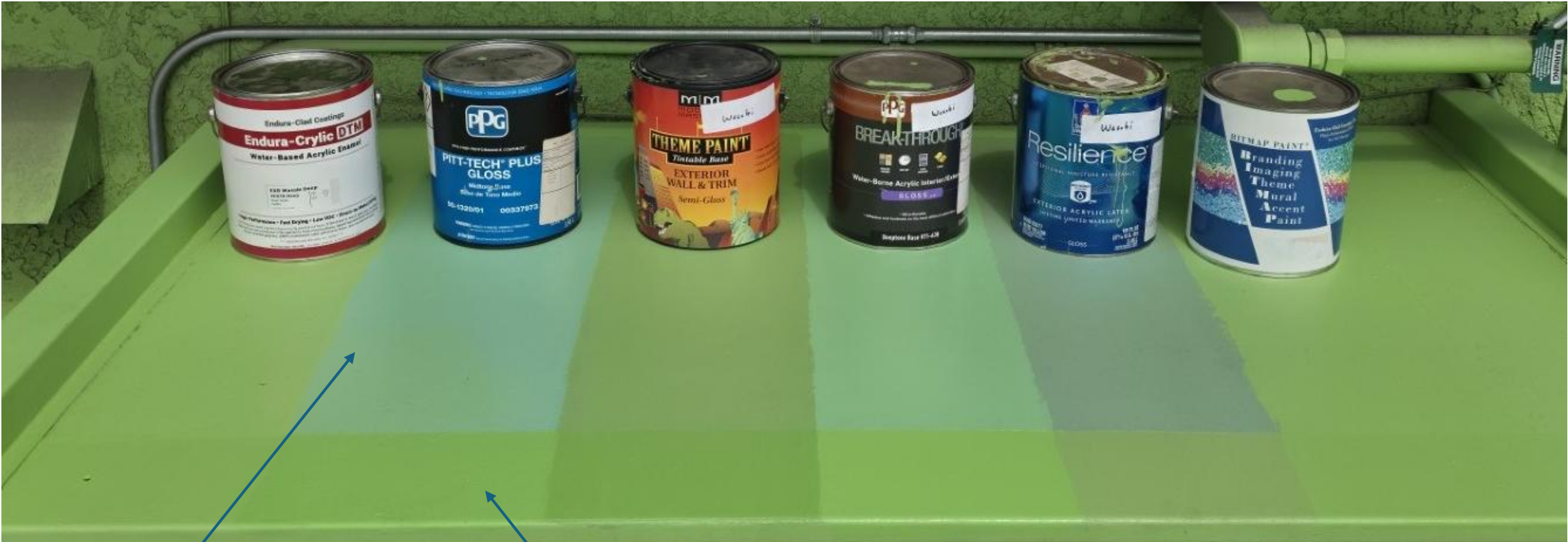
Original paint applied in June-2022 Same paint/batch re-applied May-2026. The discrepancy in color between the two is the degree of fading
